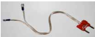
Strip ends of wires and attach plug then crimp female terminals on opposite end of wire.
